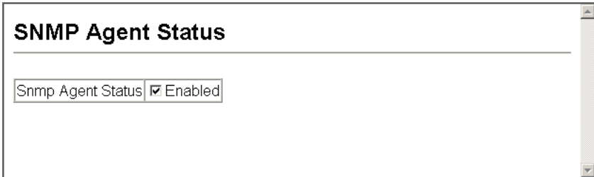
Figure 3-26 Enabling SNMP Agent Status
